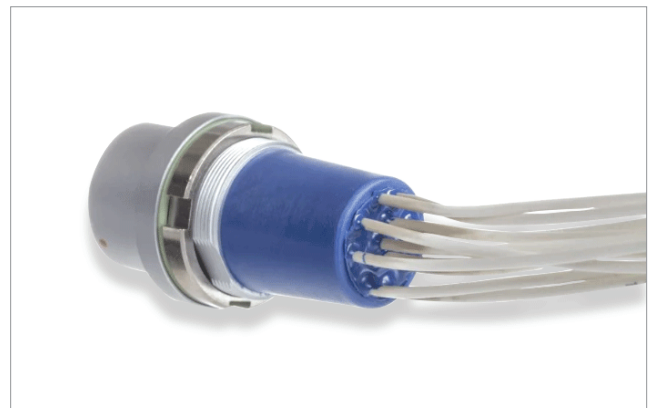
Hermetic push-pull connector with integral wires with water-blocking bond added to Teflon wire insulation.
